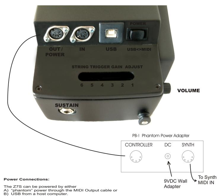
To connect to a MIDI system, attach a MIDI cable [make sure the cable has all five wires connected from end-to-end] from the MIDI Out port on the Z7S to the "Controller" port on the PB-1 Phantom Power Adapter. Press the power switch in the MIDI direction to
